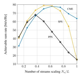
FIGURE 3. Outer layer methods at fair scattering (L = 32 paths).
