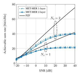
FIGURE 10. MET-MER benchmarking at poor scattering (L=8 paths),  $M_t=M_r=4$ , U=2 users and SNR = 20 dB.
