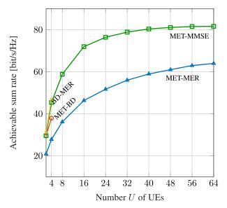
FIGURE 7. Inner layer methods at poor scattering (L = 8 paths),  $M_t = M_r = 4$ ,  $N_S = 1$  stream per user and SNR = 20 dB.
