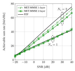
FIGURE 12. MET-MMSE benchmarking at poor scattering (L=8 paths),  $M_t=M_f=4$ , U=2 users and SNR = 20 dB.
