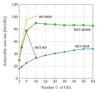
FIGURE 8. Inner layer methods at fair scattering (L = 32 paths) and  $M_t = M_r = 16$ ,  $N_s = 1$  stream per user and SNR = 20 dB.
