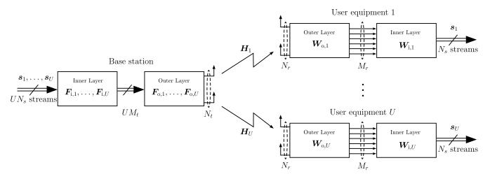
FIGURE 1. Illustration of the considered multi-layer double-sided massive MIMO system model.
