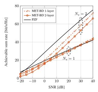
FIGURE 11. MET-BD benchmarking at poor scattering (L = 8 paths),  $M_t = M_T = 4$ , U = 2 users and SNR = 20 dB.
