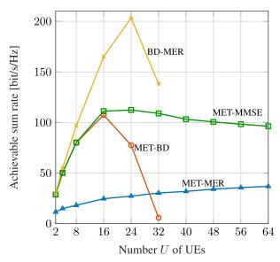
**FIGURE 9.** Inner layer methods at rich scattering (L = 64 paths) and  $M_t = M_r = 32$ ,  $N_s = 1$  stream per user and SNR = 20 dB.
