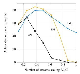
FIGURE 4. Outer layer methods at rich scattering (L = 64 paths).
