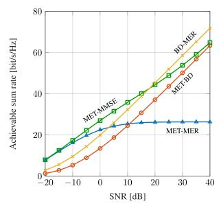
FIGURE 5. Inner layer methods at poor scattering (L=8 paths),  $M_t=M_r=4$ ,  $N_s=1$  stream per user and U=4 UEs.
